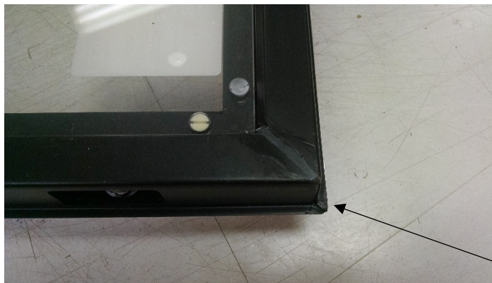
Example of welded joint repair
