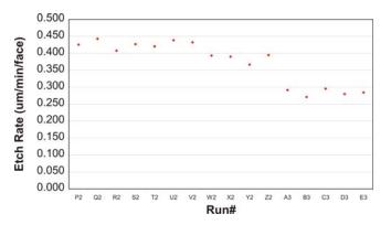
Figure 7: ER over time without dynamic feed/bleed and ICE controls.
