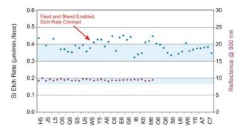
Figure 6: ER and reflectance over time with dynamic feed/bleed and ICE controls.
