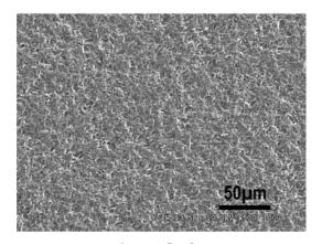
As-cut Surface Fig. 1A: Si Surface before Texturization.
