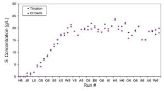
Figure 4: Concentration of dissolved Si under real time processing.
